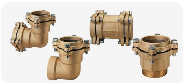
The fitting is made up of two brass parts: an EPDM 'O' ring, a catch for the 'O' ring, a compression ring and a stainless steel interior, which provides greater robustness to the pipe/fitting transition area.
