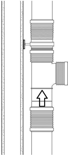
12. Finalise the installation of the fixed-point bracket or install a tensile resistant clamp on the repair socket to ensure no movement.
