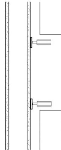
4. Install a short piece of temporary pipe halfway onto the repair coupler to secure a correct positioning of the rubber seal.
