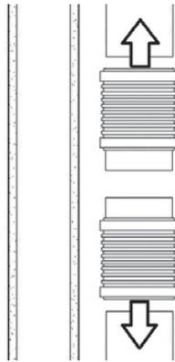
4. Secure that the pipe (or pipe and Branch) has the same length as the part which has been cut out.
