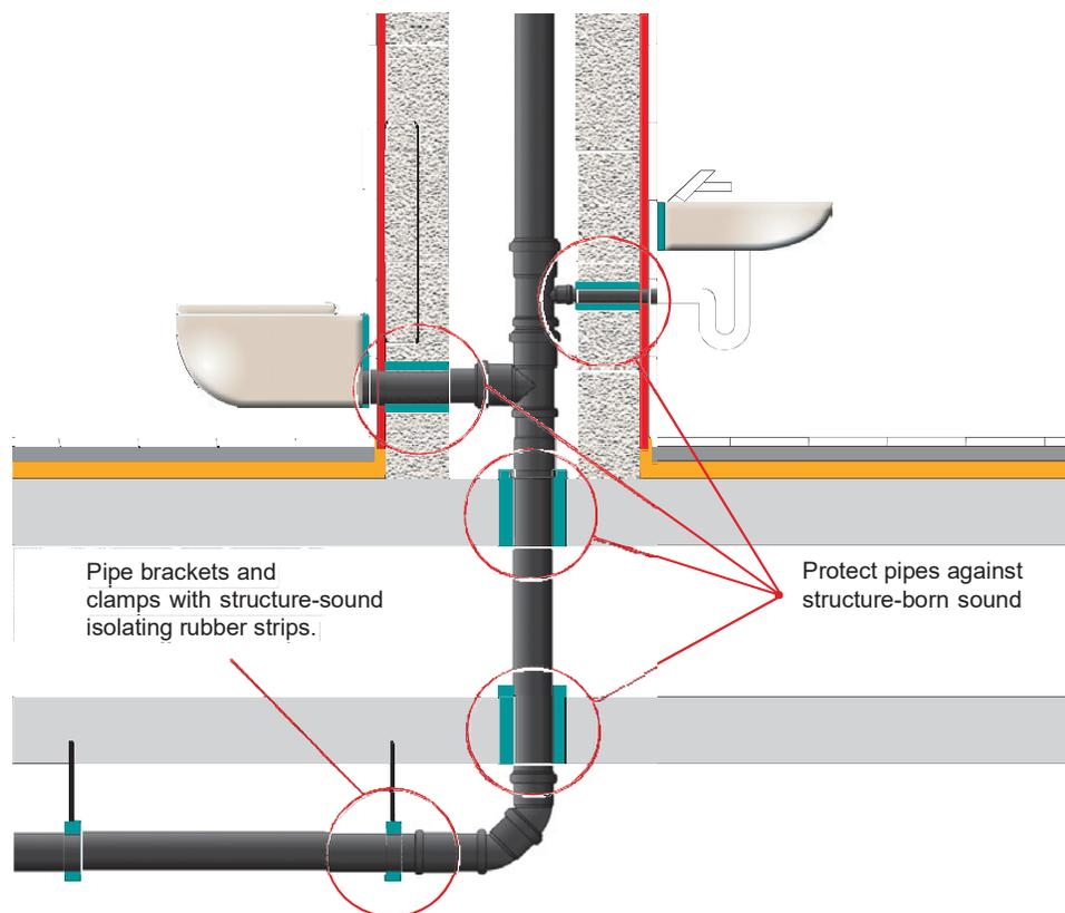
Fig. 7: Sound insulation of waste water systems.
