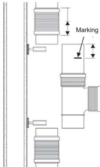
6. Install as close as possible to the two pipe ends wall plates for the fixed-point brackets and mount the threaded rod and back part of the brackets. When fixating the repair couplers with tensile resistant clamps this step can be skipped.
