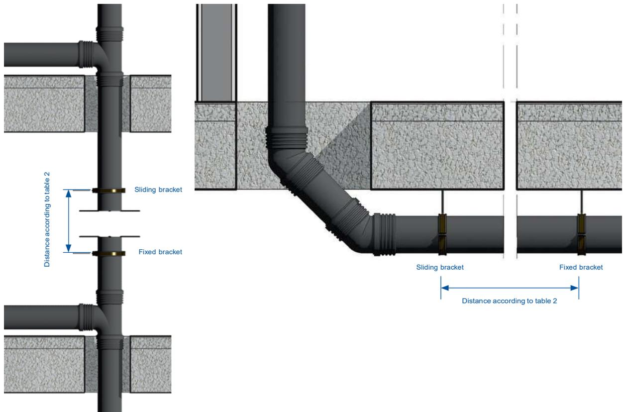
Fig 9: Example horizontal and vertical installation.
