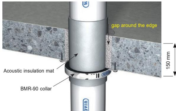
Fig. 21: Straight installation with / without sleeve / socket.
