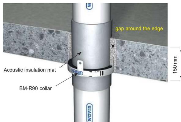
Fig. 17: Straight installation with / without sleeve / socket.
