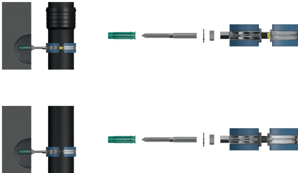
Fig. 10: Low noise bracketing – 21dB(A).
