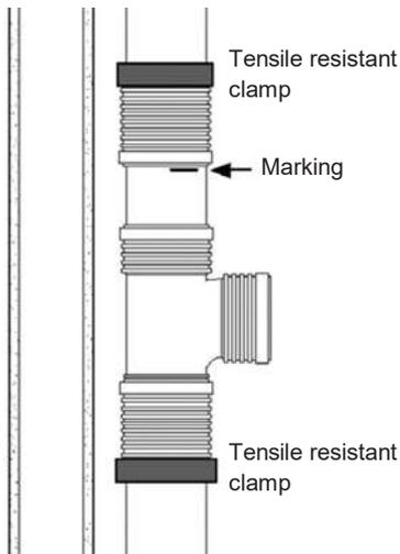
1. When inserting a branch at a later stage, please secure that the level of the branch is located at the right height. The Z1 value is mentioned for each Branch in the product overview.
