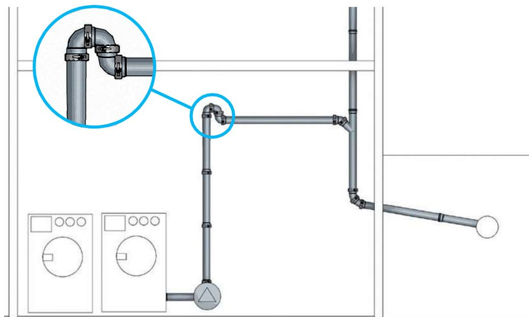
Fig. 12: Tensile resistant connection.
