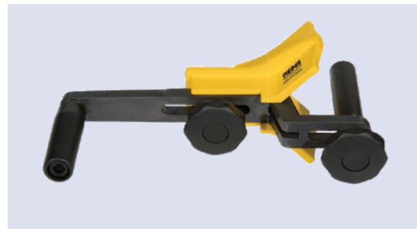
For connections to Wavin SiTech+ fittings or sockets the pipe end needs to be chamfered. Its is recommended to chamfer over a length of 5 mm under a 15 degrees angle. This can be done by using standard chamfer tooling.
